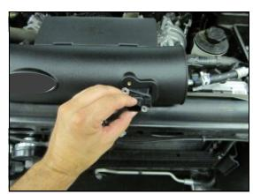
7. Transfer the MAF sensor into the Airaid Intake Tube (#2) and secure using two 8-32 x 3/8" button head screws (#11). **Do Not Use The Factory Torx Head Screws!**
