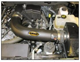
**8. A.)** Insert the Airaid Intake Tube into the couplers as shown. Check for alignment, and tighten all clamps. **B.)** Re connect the Mass Air Flow Sensor. Apply the Airaid Bubble Decal onto the Intake Tube as shown.
