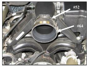
**6.** Install the Silicone Coupler (#6), one #64 Hose Clamp(#14), and the #52 Hose clamp (#13) onto the engine air inlet. Leave the clamps loose for now.
